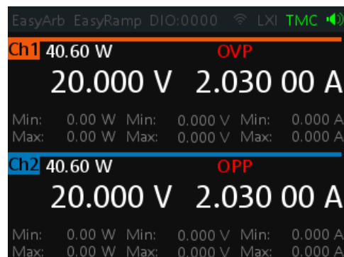
Figure 7-14: Indicator of OVP/OPP when tripped
