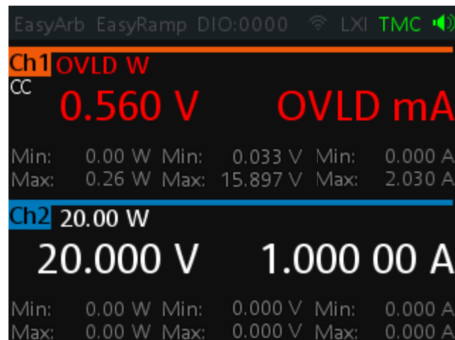
Figure 7-6: Display of OVLD indicator when current > 205 mA at Ch 1
